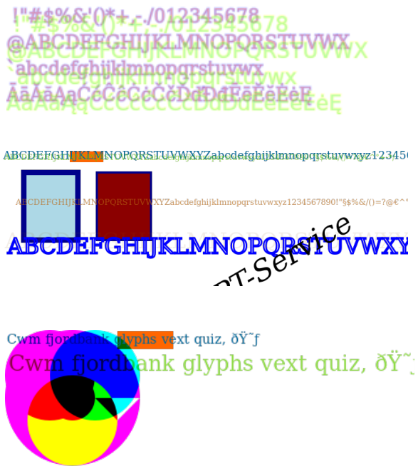
Figure 11: Sample canvas fingerprinting images. These three images represent the final canvas images created by fingerprinting scripts, which are subsequently hashed and used to identify the device.
